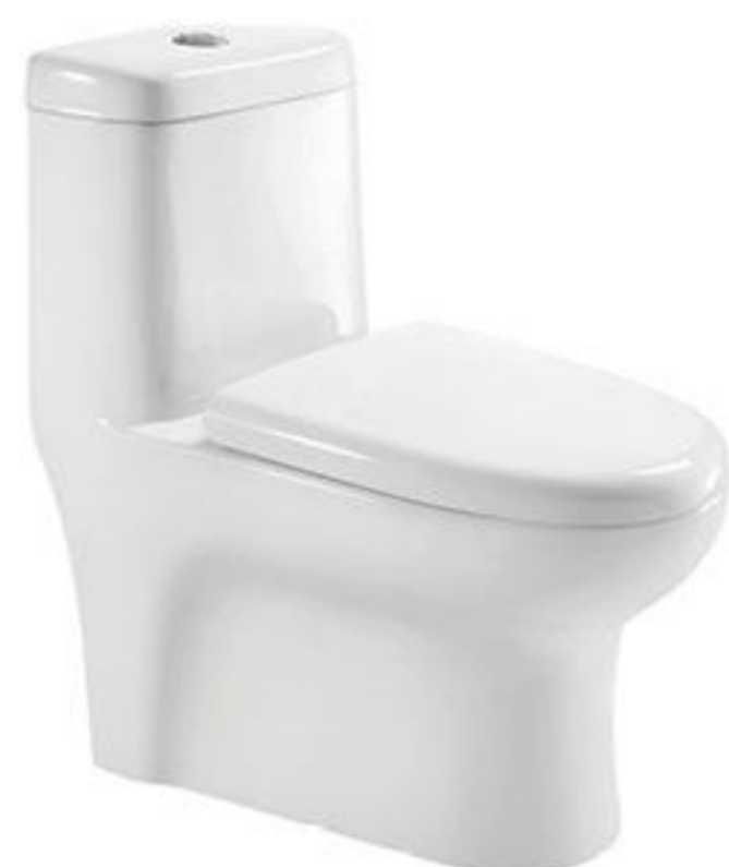
8249 Siphonic One-piece Toilet Size: 680x380x780mm S-trap: 300/400mm Roughing-in
