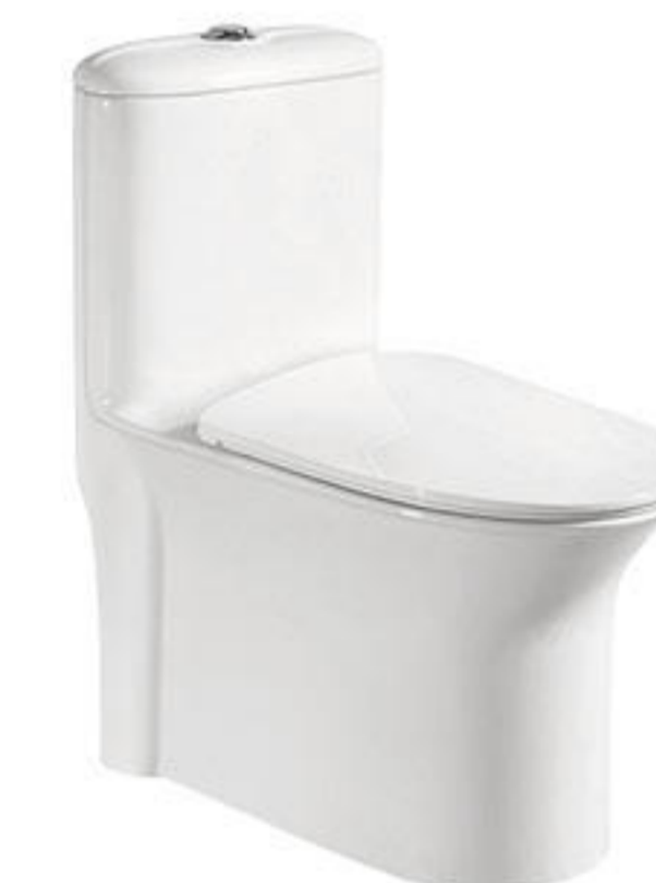
821 Siphonic One-piece Toilet Size: 665x360x750mm S-trap: 300/400mm Roughing-in
